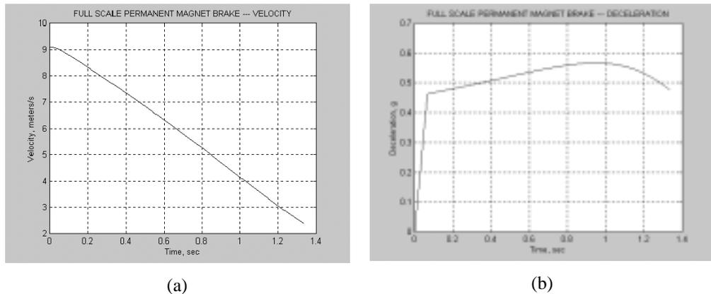
*Figure 5. Prediction for full-scale magnetic brake. (a) Velocity. (b) Deceleration*
