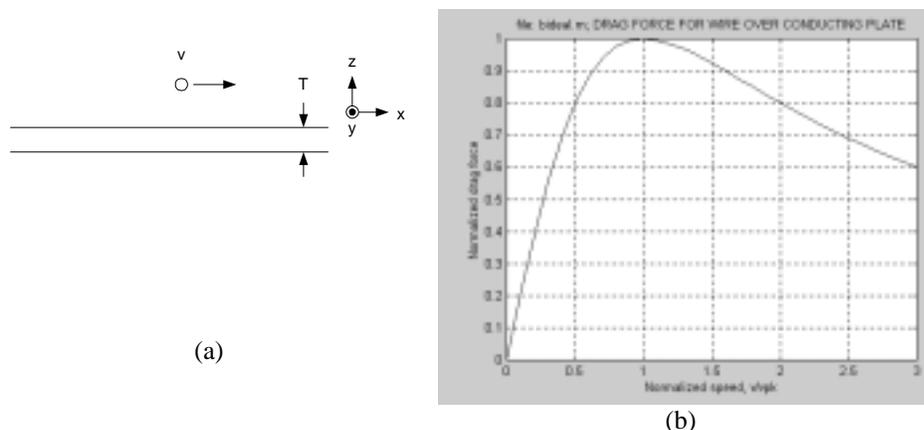
Figure 1. Current-carrying wire traveling over a stationary conducting plate
