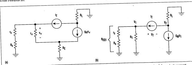
3. THE RESISTANCE FACING  $C_{\mu}$  with  $C_{\pi}$  open-circuited is even more difficult to calculate. Applying a test current source across the  $C_{\mu}$  terminals yields a complicated result (a). It's better to replace the equivalent resistance at node  $V_1$  by a resistance  $(R_1)$  that accounts for the transistor's input impedance, and to substitute an equivalent dependent source  $(G_M V_1)$  for the  $g_m v_{\pi}$  generator.
