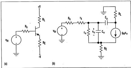
1. THE MOST GENERAL TRANSISTOR AMPLIFIER has a source resistance, an emitter resistance, and a collector load resistance (a). The circuit's small-signal model substitutes resistors and capacitors for the transistor (b).
