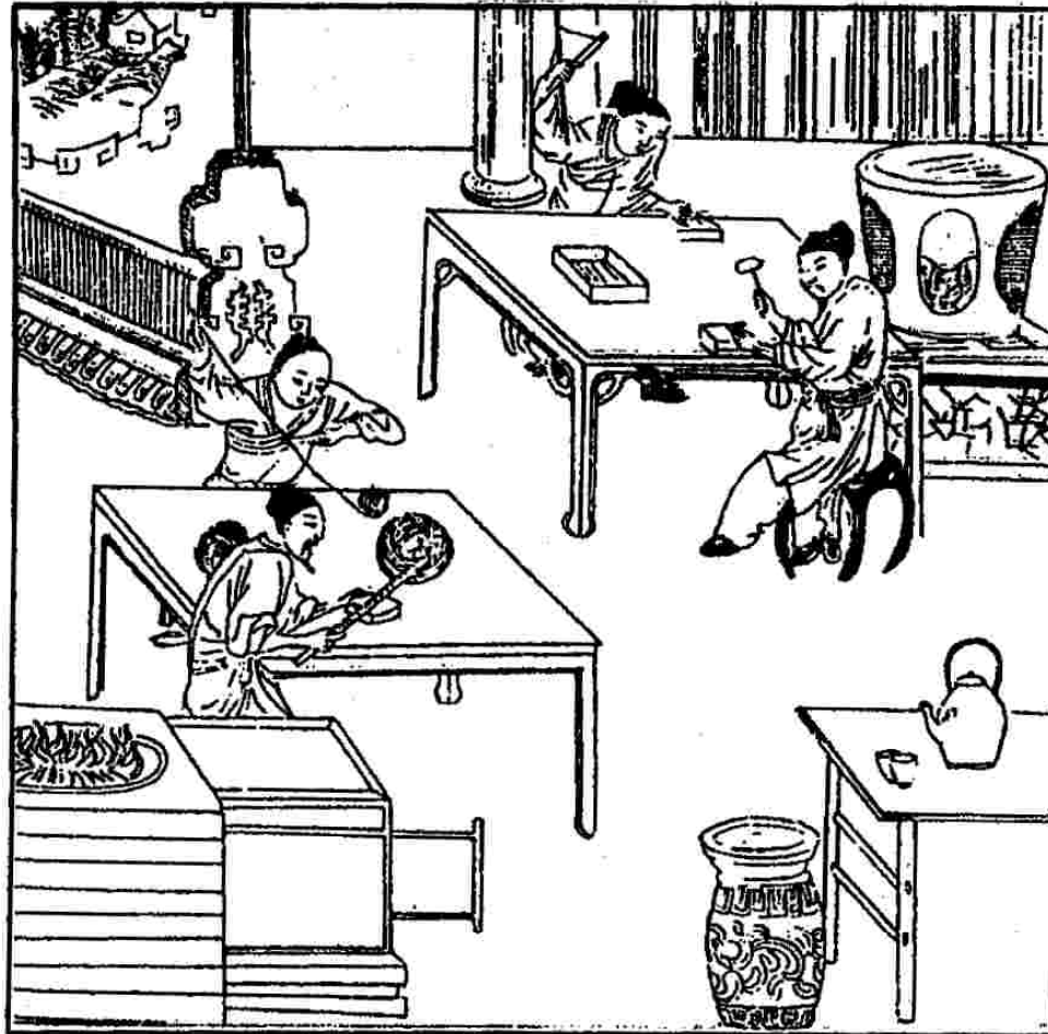
Figure 1.1 Magnetic needles for compasses are being made by craftsmen in this print of 1637. Good steel was manufactured in China from 500 A.D. onwards.
