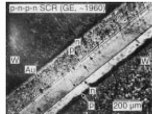
Fig. 7. Cross section of an early (1957–60) GE Si p-n-p-n SCR, with Ga diffused p-type regions) into both sides of a \sim 250 \mu\text{m} n-type Si wafer and with an n-type emitter regrown on top from a Au (+Sb) alloy.
