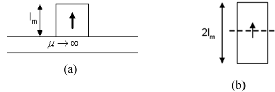
Fig. 3. Method of images. (a) Permanent magnet on top of a piece of steel. (b) Equivalent circuit using method of images for prediction of magnetic field above the steel surface.
